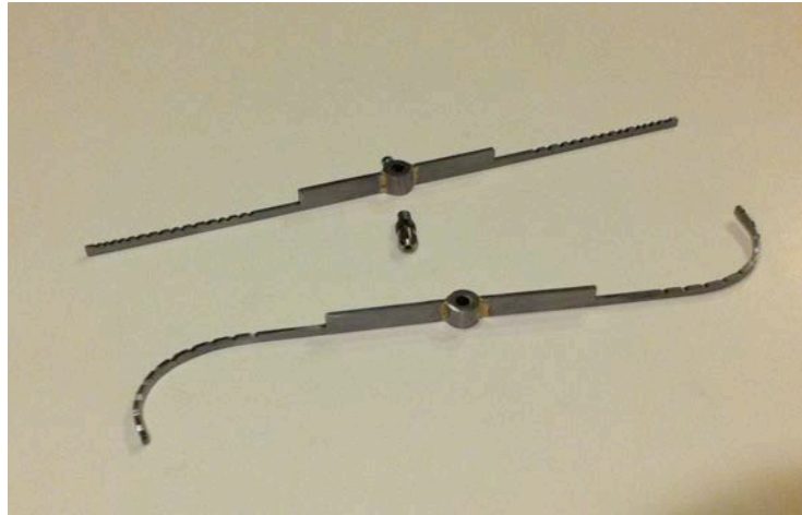
Fig 12 Model sinous foliot and replica of Llanthony foliot for testing at the BM.
