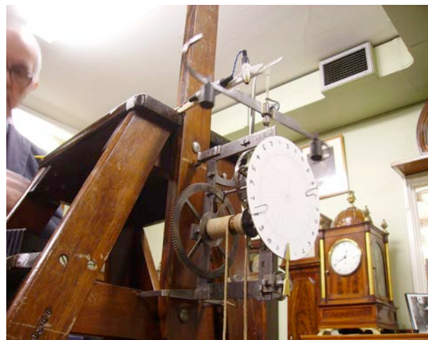
Fig 13 Hammond clock in the British Museum fitted with sinous foliot. Compare with the pictures of the intarsia panels.
